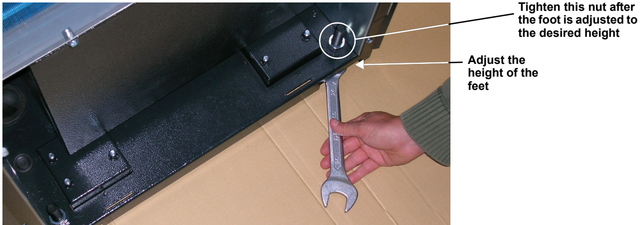
Figure 12 Adjust leveling feet
